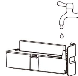
5. Add about 1L cold water through the inlet, filling around 80% of the water tank.
