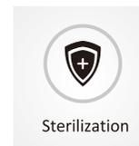
When the machine is on, pressing "sterilization" button will turn on UV sterilization mode, and pressing one more time will turn it off. (The icon will stay on when the machine operates in sterilization mode, otherwise it will be off.)
