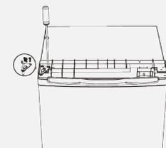
25. Place the cover plate in position and secure it at the rear with the two screws.
