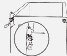
20. Insert pin of the upper hinge in the fixture of the upper appliance door.
