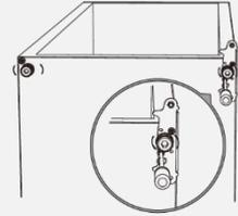
15. Release the pin from the lower hinge, turn the hinge 180° and reinsert the pin.
