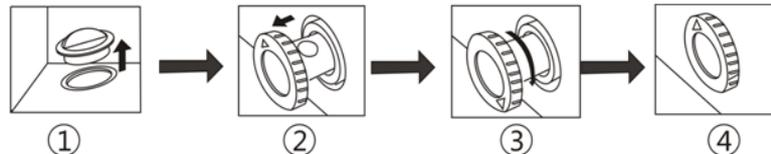
6. To drain the condensation water, place a collection container under the condensation water drain (at the bottom of the front of the appliance).
