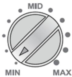
**Temperaturregler Gefrieren / Freezing temperature controller**
