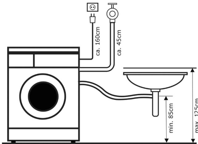
Connect to the water tap using the hose supplied by the manufacturer. Connect the bent end to the back of the appliance and the straight part to the tap.
